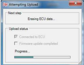
To begin the upload process, simply choose the COM port to which the ECU is connected (the software will tell you which ports are currently active) and then click 'Start Update'. Now turn on the ignition. The firmware upload takes approximately fifteen seconds, after which the ECU is ready to use. (Shown above right).
