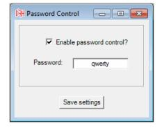
If you have forgotten the password or would like to force entry into a previously locked ECU, this is also possible, although all settings in the ECU will be completely removed.
