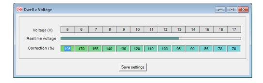
When the supply voltage drops below 12v, a coil will take longer to charge and therefore the percentage correction should be greater than 100%. The opposite is true when the voltage is higher than 12v. The correction should always be set to 100% at 12v.
