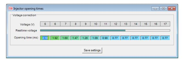
For each possible voltage, there is a programmable opening time (in ms). Most injectors have an opening time of between 0.8 to 1.0 milliseconds at 12V. Injector opening times can be specified to the nearest 64 microseconds.
