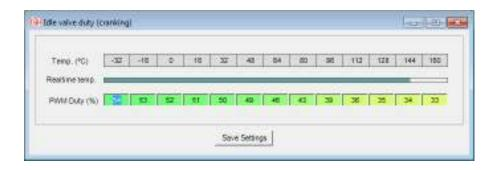
When starting the engine, we also need to specify the quantity of air that is required. This is governed by the idle control valve. In cold temperatures, more air is required to provide a higher engine speed. To access the settings for the idle control valve when cranking, click 'Cranking/startup > Idle valve setting'.
