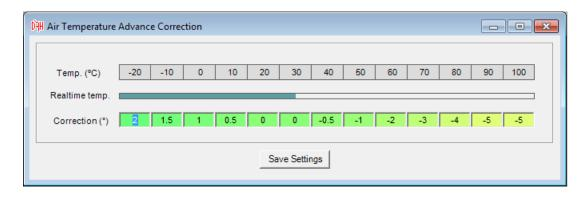
It is possible to specify ignition advance correction in 0.5 degree increments, which will act on top of the advance figure calculated from the main ignition maps. In the example above, an ambient air temperature of fifty degrees Celsius would reduce the total amount of ignition advance by one degree.
