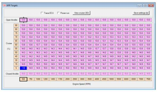
It is important to remember that the oxygen sensor is relatively slow to react to changes in AFR. Therefore, an oxygen sensor should never be relied upon to provide accurate fueling when an engine is under full load. Instead, set the closed-loop feedback to activate when certain conditions are met.
