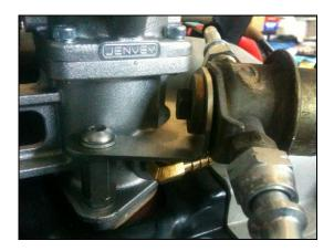
The fuel pressure regulator bracket & crank sensor brackets are attached under the manifold bolts on cylinder number three:
