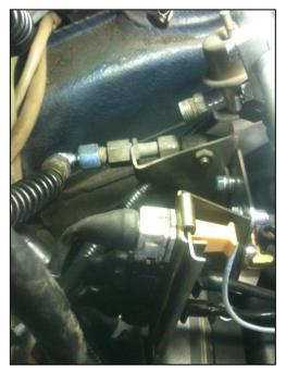
Use the ninety degree male to female adaptor to attach the fuel return hose to the fuel pressure regulator (as shown to the left). This prevents the hose from bending too far which could cause a kink / blockage.
